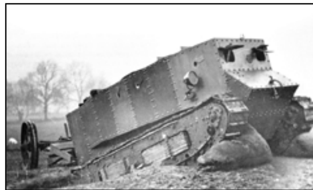
PROTOTYPE: “Little Willie” was the first prototype tank. It carried a crew of three and could travel as fast as 4.8 km/h.
